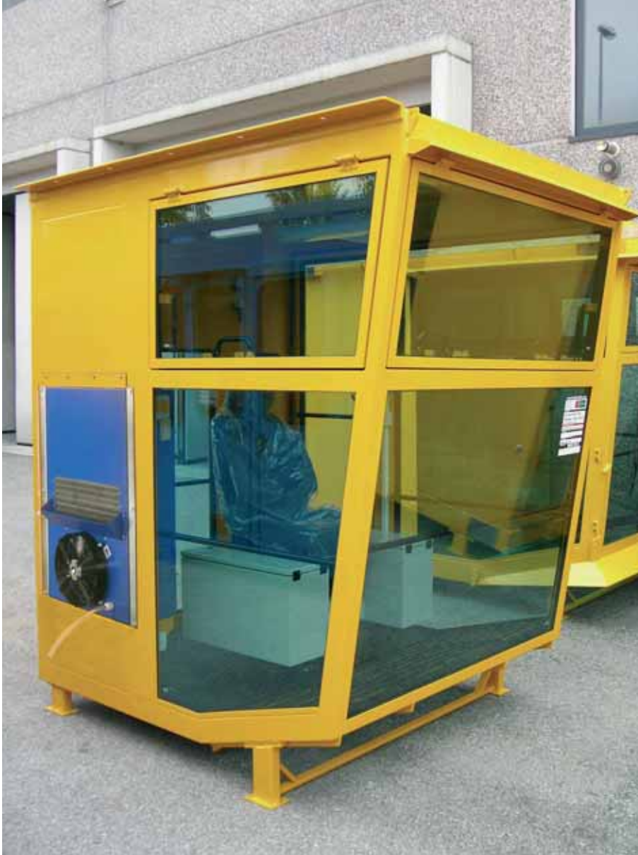
Wall Air Conditioner installation
